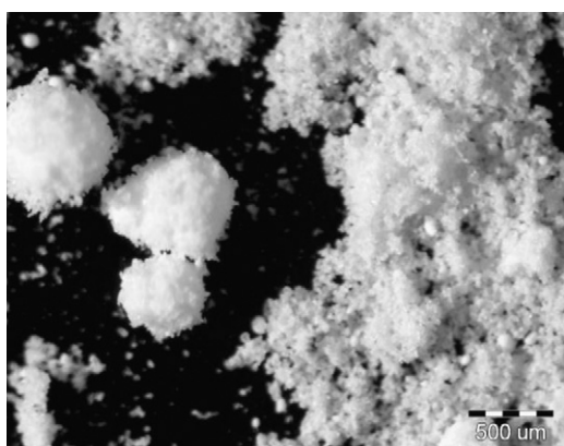
Fig. 8. Immersion as a predominant process in nucleation phase in case of Lutrol® F68.
